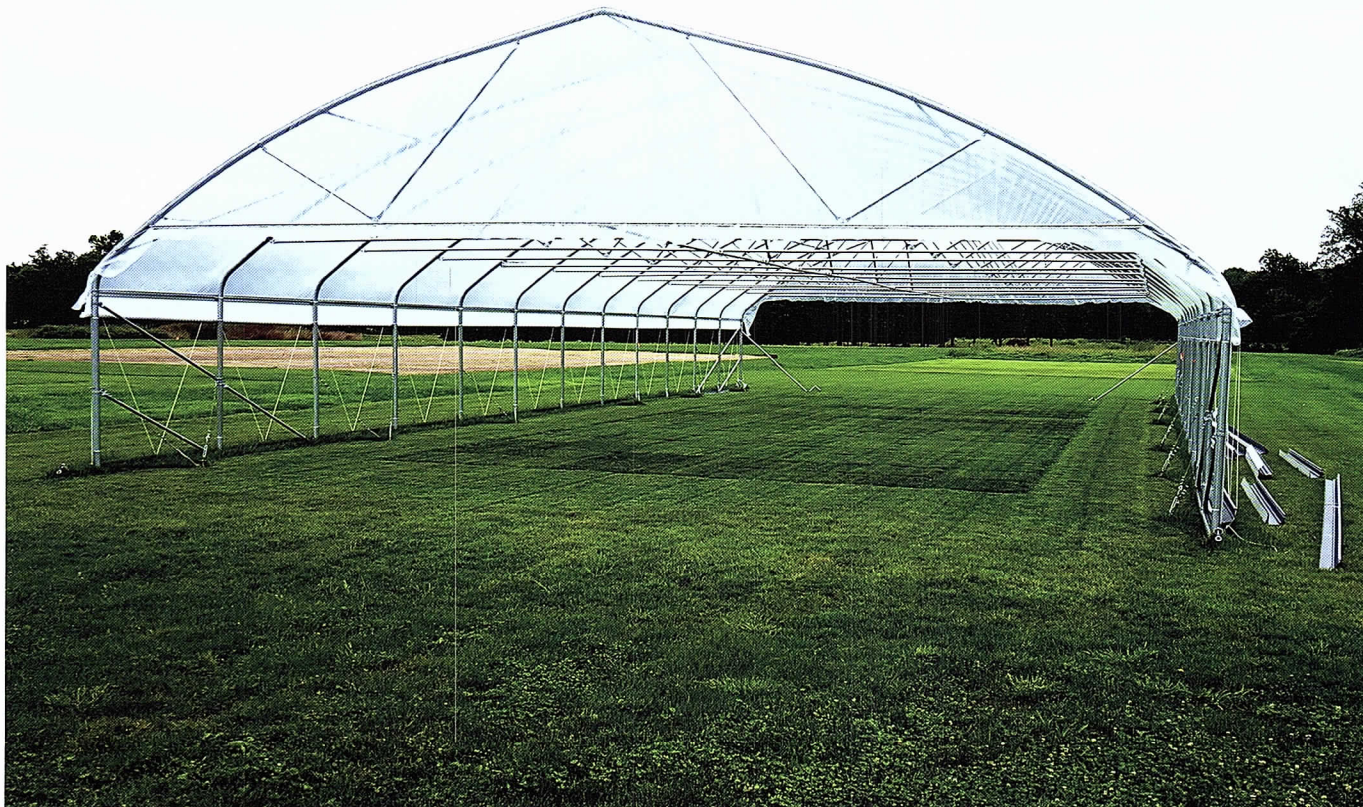
Cool-season drought shelter at College Park, MD, before initiating drought on USGA/NTEP Cool-Season Water Use Trial.
